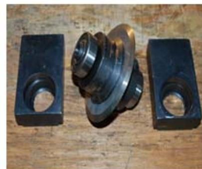
17. put the bearing back in both side block
