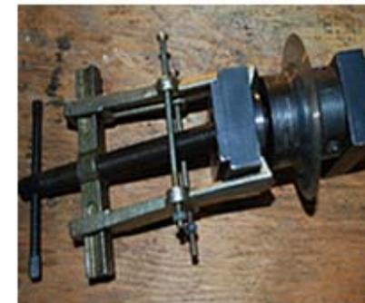
**12. use puller to separate the side block and bearing on both side**
