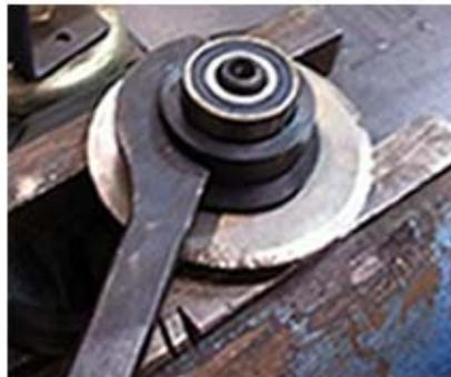
14. use hook spanner to loose the fasten nut
