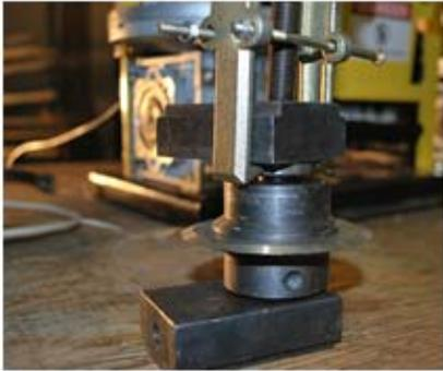
12. continued-- use puller to separate the side blocks and bearing
