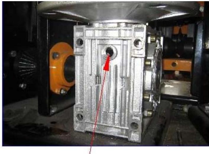
**Fill up with high performance gearbox or motor oil**
