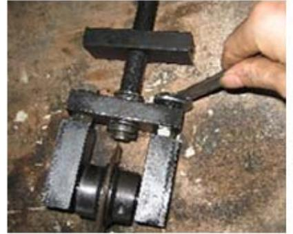
18. use screw to put the blade assembly back together
