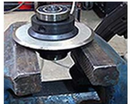
13. use machine vise lock one side of fasten nut
