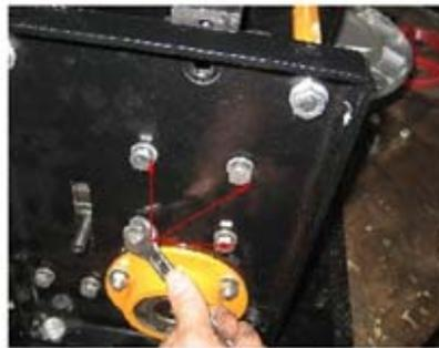
**8. LOOSE the lead rail on both side**
