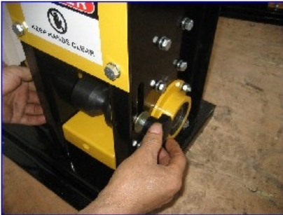
1. unscrew the hand lever
