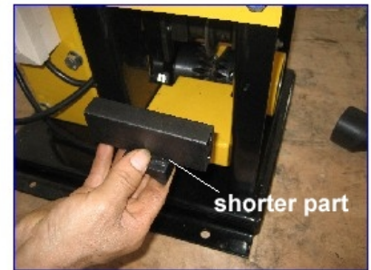
3. insert the square spindle shorter part at front
