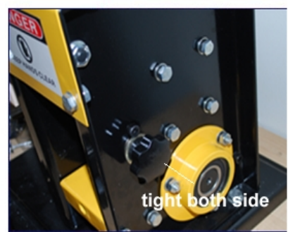
6. tight the hand lever tight both side
